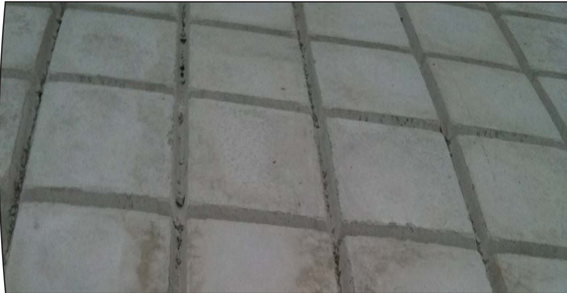
FLEXICRETE® panels are 2.3m x 3.6m comprised of 400mm x 400mm x 81 mm thick concrete blocks connected by galvanized wire mesh
