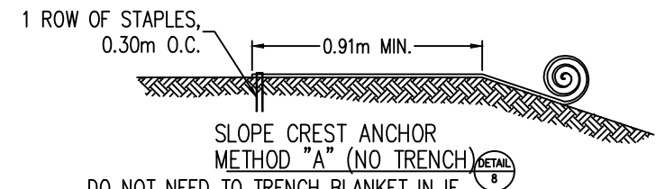
SLOPE CREST ANCHOR METHOD "A" (NO TRENCH) (DETAIL 8)
