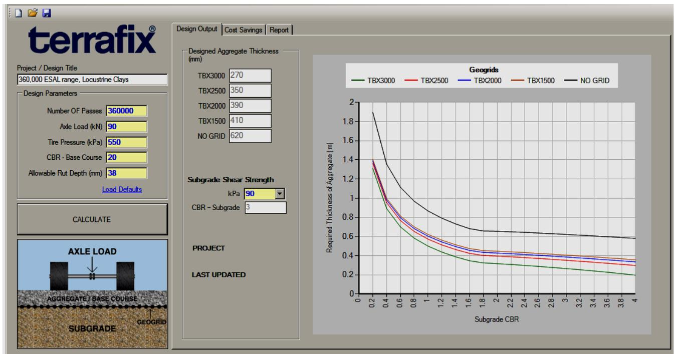
The following equivalent aggregate thicknesses can be determined for this particular set of conditions:
