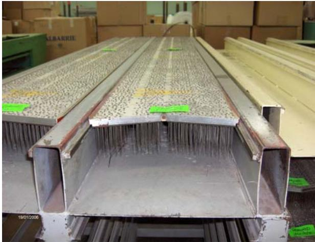
Figure 6. Needle-punching board.
