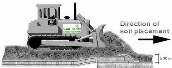
Figure 3. Schematic soil placement over a GCL
